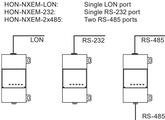
TONN9 supports up to four expansion modules and they may be installed in any combination up to the maximum permitted number for each module type:
