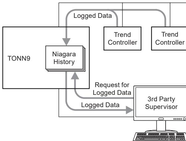
In the diagram above the TONN9 has been configured to archive the logged data from the Trend controller(s). This data is regularly archived by the TONN9 and stored in a Niagara history. When the logged data is required by the 3rd party supervisor, it requests the data from the appropriate Niagara history in the TONN9. The data is then passed from the TONN9 to the supervisor where it can be processed as required, e.g. to display a graph of the data.
