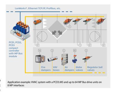
nication driver FBox and can then exchange data with the application program via the respective FBoxes. The Belimo components are generally commissioned from the application program using the SBC FBoxes. Only a few components such as VAV controllers require additional Belimo parameterisation tools to adjust their operational parameters.
