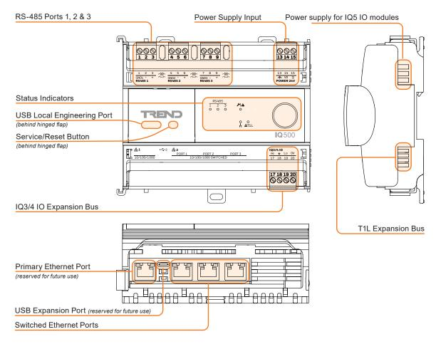
Note: An RJ-11 socket is located on the left hand side of the IQ500 and is reserved for future use.
