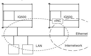
In addition, the IQ500 has the ability to join an internetwork using its virtual internetwork node controller (vINC).
