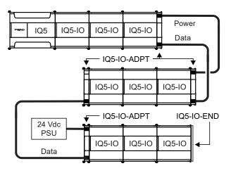
A protective cover (IQ5-IO-END) is supplied with the IQ500 to protect the T1L contacts when not in use. This can be removed and fitted to cover the contacts of the last module on the T1L bus. Spare covers are also available.
