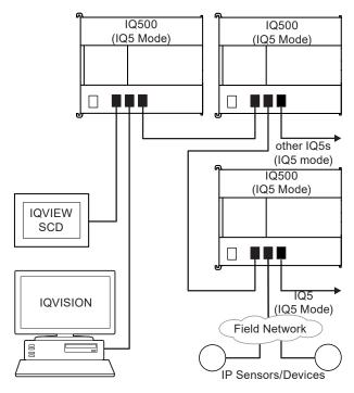
Using one of the ports the IQ500 can form a Trend LAN with other IQ5-compatible devices over an Ethernet network:
