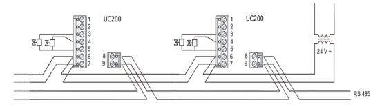
Connection of power, communication, and valve. Suitable cable types are LAM DATAPAR 2×0.8 (cross-section in mm²), JYTY 2×1 (diameter in mm) etc. If communication and power are in the same cable, use 4-core LAM DATAPAR 2×2×0.8, JYTY 4×1. Up to 100-120 meters,
